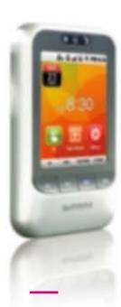
Max user: 200,000 Image Log capacity: 1,000,000 Face log capacity: 5,000 CPU: 667 MHz RISC LCD: 3.5" touch screen Memory: 1GB flash + 128MB
