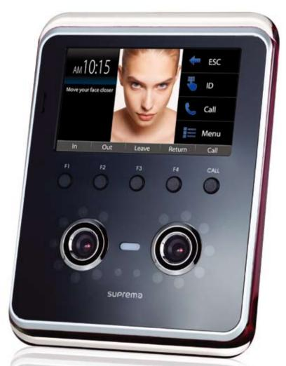
1,000 matches in 1 second (1:N) User capacity: 1000 (1:N), 10,000 (1:1) Log Capacity: 1,000,000(event), 10,000(image) CPU: 1.1GHz DSP, 667MHz RISC LCD: 4.3" WVGA Touchscreen
